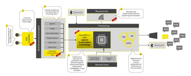
Figure 4. Diagram of BiCore processing pathway.
