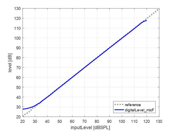
Figure 2. Input/Output curve for microphone + analog/digital converter showing linear performance up to 117 dB SPL input.
