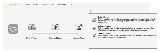
Figure 3. SoundPro 2.0 software interface to adjust the balance between speech and background noise.
